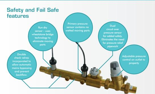
**Dual circuitry** The system controller incorporates a number of safety features. As well as the primary pressure sensor there are two other sensors. These provide RUN DRY PROTECTION and OVER PRESSURE PROTECTION.
