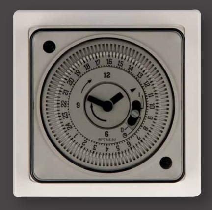
OP-SBST is a captive-tappet 24-hour time switch. Each tappet operates for 15 minutes. The timer is suitable for installation on a surface or in-wall pattress box. The 24 hour dial controls a volt-free changeover switch, with a resistive rating of 16 amperes.
