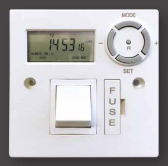
The OP-DFST is a digital fused-spur time switch. The timer is suitable for pattress box mounting. The 7 day programming logic controls a mains-linked switch, with a resistive rating of 13 amperes. There is an inbuilt rechargeable cell to keep the timer running in the event of a loss of mains power. The output can be disconnected by an integrated double-pole isolator switch; the load is protected by a replaceable BS1362 13 Ampere cartridge fuse, within a removeable caddy.
