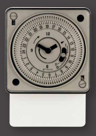
OP-TS111.1 is a captive-tappet 24-hour time switch. Each tappet operates for 15 minutes. The timer is suitable for surface, panel and din-rail mounting. The 24 hour dial controls a volt-free changeover switch, with a resistive rating of 16 amperes.
