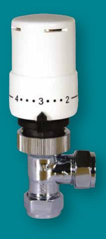
Thermostatic valves are typically used for regulating the fluid flow to the radiators of central heating systems. They are provided with a regulating element which automatically controls the opening of the valve to keep the ambient temperature of the room where they are installed constant at the set value.
