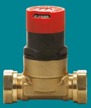
The Tower auto bypass valve (ABBV1) should be fitted where a boiler bypass is required – typically this is the case when a system is equipped with thermostatic radiator valves (TRV's), and to allow pump overrun operation after zone valves have closed down.
