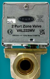
The VAL222MV is a 2 port spring return zone valves with 22mm compression fittings and an auxiliary switch. This is for general purpose flow control applications or central heating systems. When correctly wired with an appropriate room thermostat, cylinder thermostat and programmer the valve will control the water flow from the boiler to hot water and from boiler to central heating.
