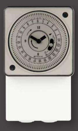
OP-IHTGPT is a 24 hour immersion heater time switch, suitable for surface mounting. The timer controls a volt-free changeover switch, with a resistive rating of 16 amperes. Pre-fitted (removable) link for mains switching.
