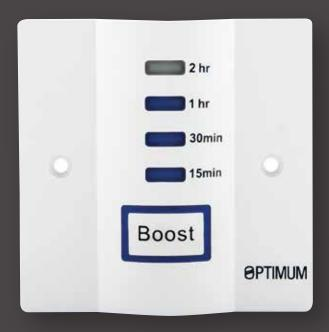
The OP-EBT2 is a two hour electronic, one-button boost timer with visual indicator. There are four pre-set timed outputs. Suitable for installation on a surface or in-wall pattress box. The electronic timer controls an internally linked output relay, with a resistive rating of 16 amps. An earth park terminal is provided. Surface-run cord outlet with cable restraint. Press up to 4x to select boost output, press again to cancel.
