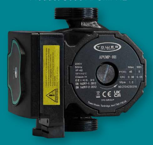
The APUMPHE is equipped with permanent-magnet motor and differential pressure controller, capable of automatically and continuously adjusting motor performance to meet the actual needs of the system. When the pump is working, the pump is controlled according to the principle of "Proportional Pressure Control (BL)" or "Constant Pressure Control (HD)." In these two control modes, the pump performance and corresponding power consumption will be regulated according to the heat demand of the system.
